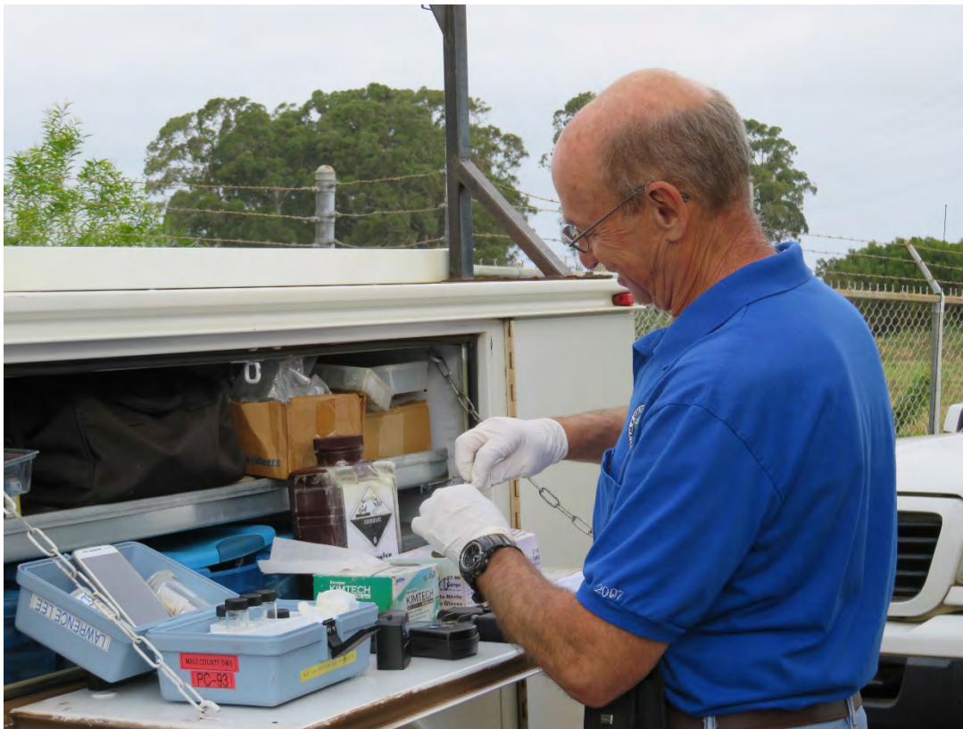
Electronic Technician Lawrence Lee performing field calibration for online chlorine analyzer.
